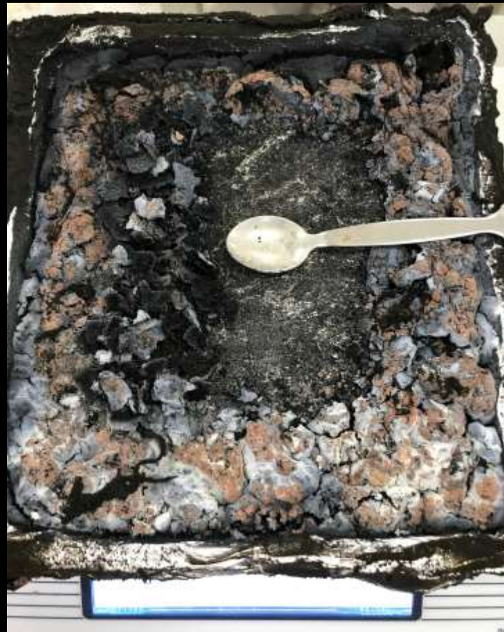
PelletPave sample after Furnace, average amount unburnt \approx 26%
