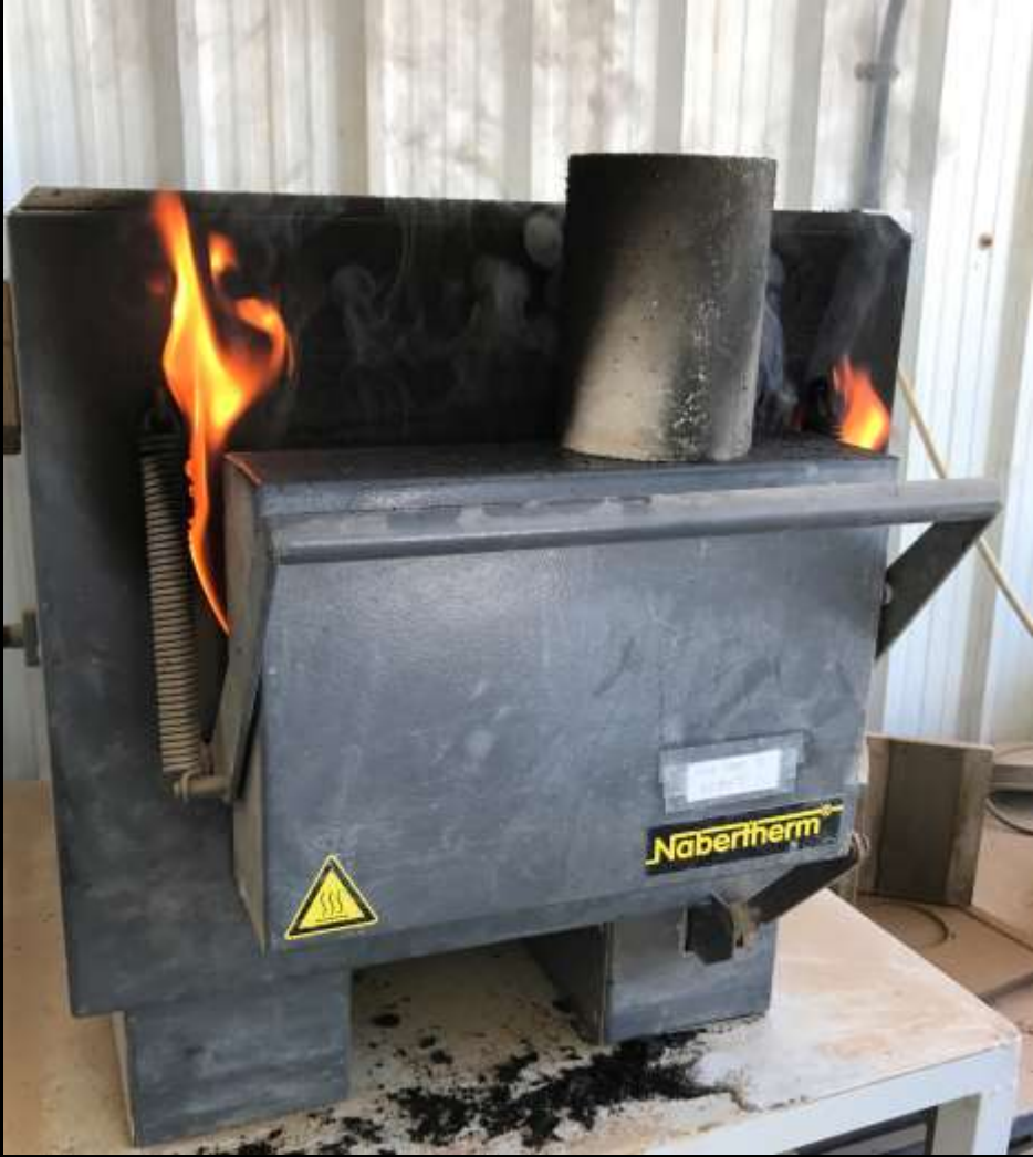
Pure PelletPave in Furnace at 540°C
